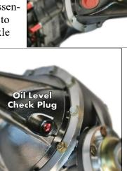
Pinion Inspection Fill Plug
